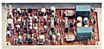
2 UNIQUE PHASE SHIFTER CIRCUIT: Included in the synthesizer decoder is a unique phase shifter circuit that gives the two rear channels a phase difference of 90 degrees each—plus 90 degrees to the rear left channel and minus 90 degrees to the rear right channel, This puts the rear channels in phase with each other, and establishes a correct phase relationship among all four channels, creating distinct sound images of original sound sources.
